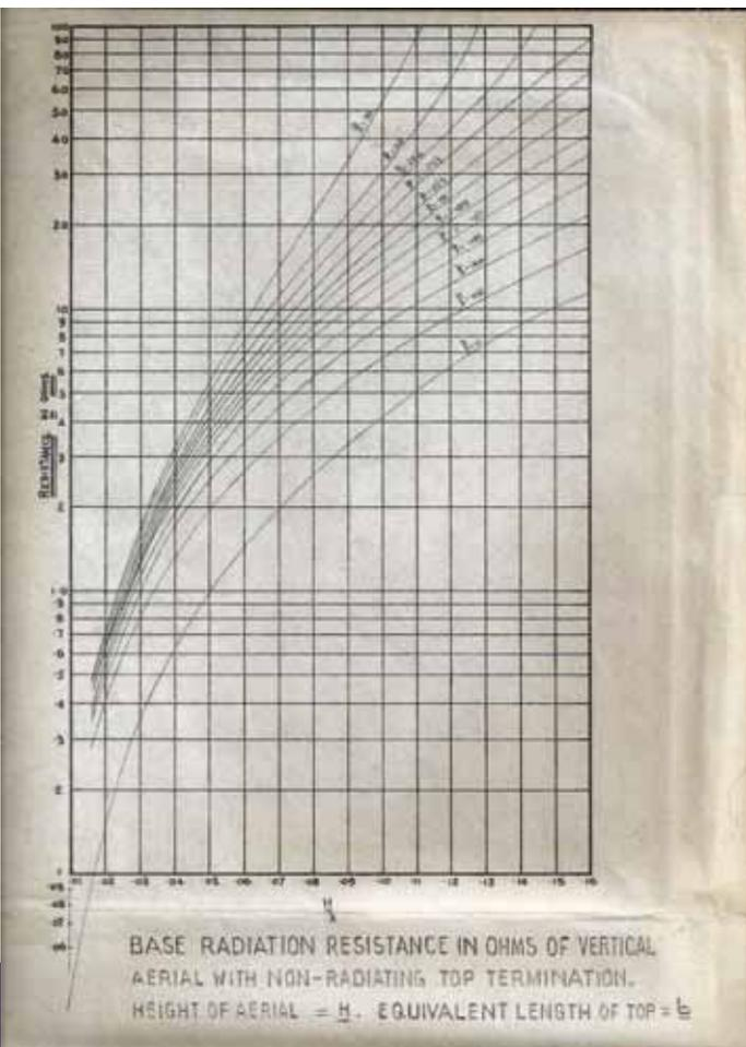
From this you will see that the Radiation Resistance of a 4m whip at 80m ( $= \lambda / 20$ ) is 1 ohm.
